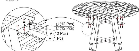
Note 1: Insert all the bolts into their respective holes half tight at first. Fully tighten only when all the bolts have been successfully inserted into their holes.
